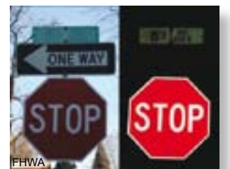
The selection of sign sheeting plays an important role in ensuring all signage is visible at all times of day.
